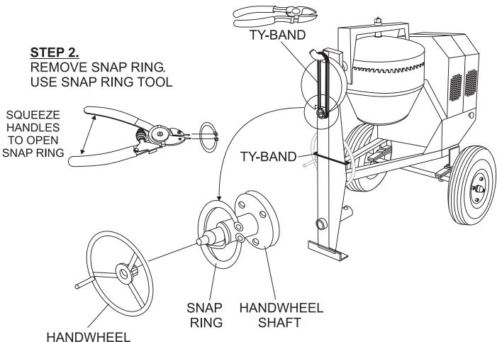
Figure 4. Handwheel Assembly
